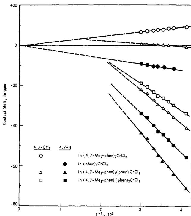
Figure 1. Temperature dependence of 4,7-CH<sub>3</sub> and 4,7-H shifts in mixed ligand complexes of (4,7-Me<sub>2</sub>phen)<sub>3</sub>CrCl<sub>2</sub> and (phen)<sub>3</sub>CrCl<sub>2</sub> in *d*<sub>4</sub>-methanol.
